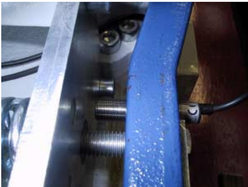
Pic. 2: showing the inductive proximity switch for the Brake Lining Wear control
